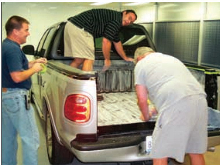
Shops should create one area where technicians remove grease and wax from the truck bed, sand it and then solvent-wipe the surface for application; and another to mask and prime the bed before coating it with the bedliner material.
