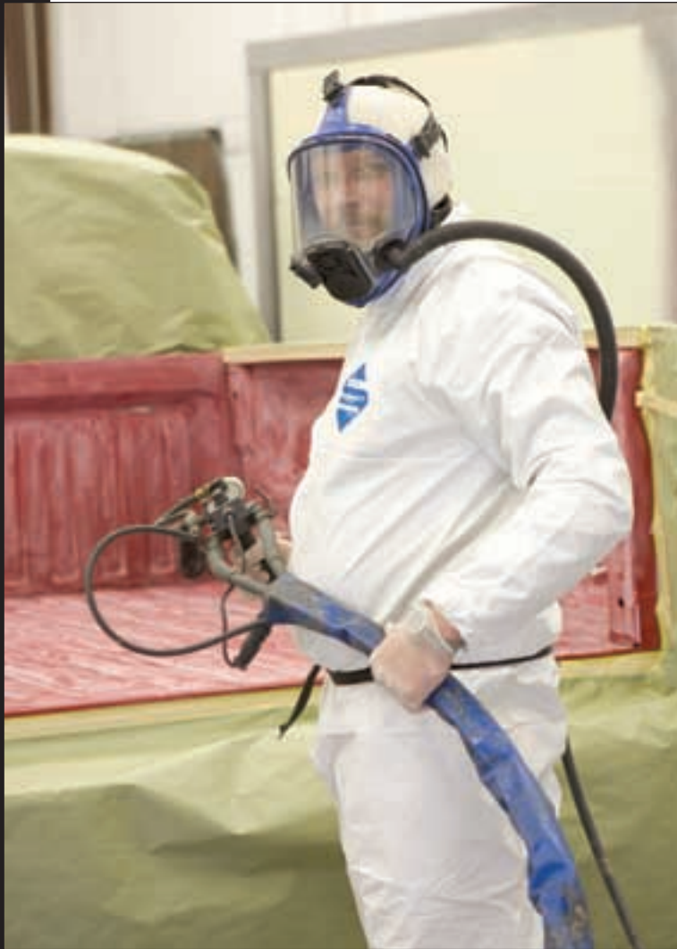
Proper safety equipment—including a head covering, face shield, paper spray suit, fresh air supply and protective gloves—is an essential part of any shop setting up to offer spray-on bedliners.
