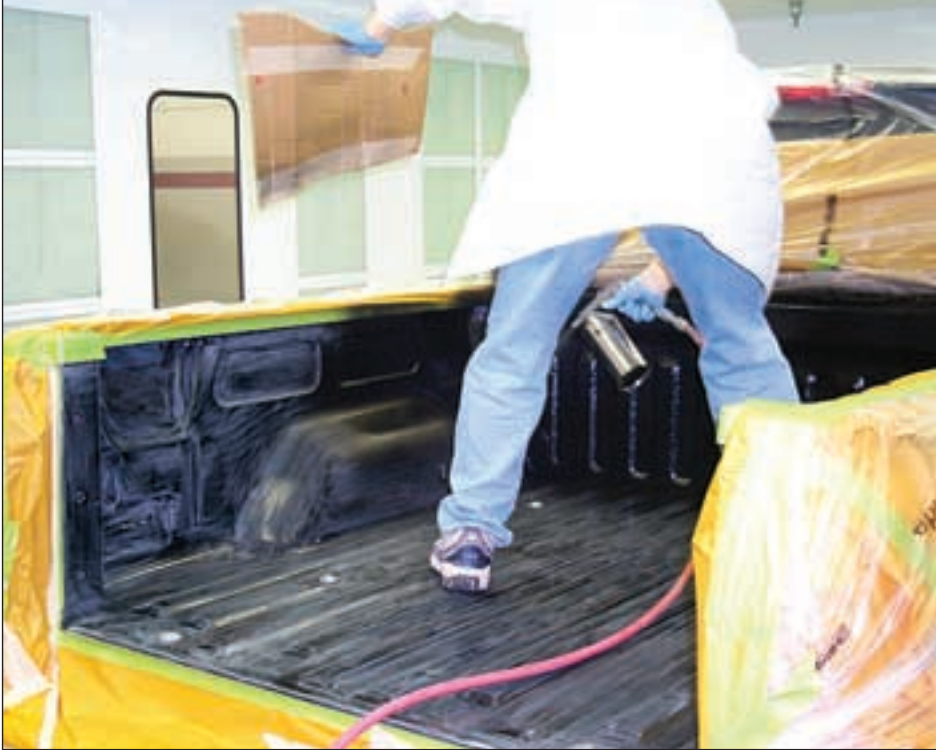
Once a vehicle has been sanded and taped-off, it can then be moved to a dedicated application area for spraying.
