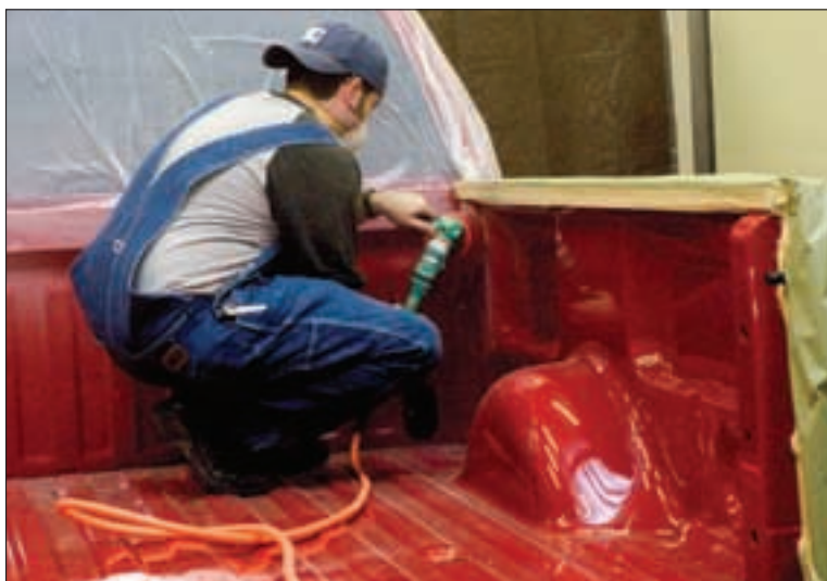
Performing prep work in a separate room ensures that sand and paint particles won’t end up embedded in the liner.
