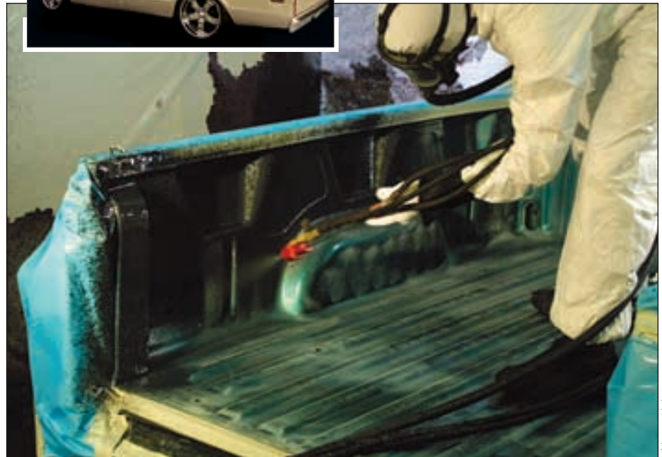
Taping plastic on booth walls and using cardboard or other disposable materials on the floor makes it much easier to clean up after a day of spraying.
